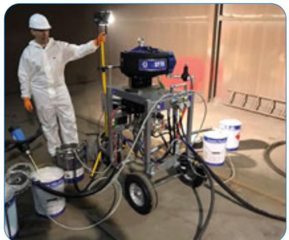
LA GAMME PNEUMATIQUE EST CONÇUE POUR FONCTIONNER AVEC UNE ALIMENTATION D'AIR, SUR CHARIOT OU MURALE, ELLE POURRA VOUS SERVIR SUR CHANTIER OU EN ATELIER
